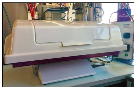
Fig. 1: The novel wave-mixed single-use SmartRocker bioreactor with Finesse G3Lab Universal Bioreactor Controller.
