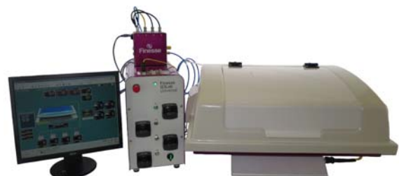
Fig. 1: Picture of the Finesse SmartRocker bioreactor with PC based Finesse G3Lab Universal controller
