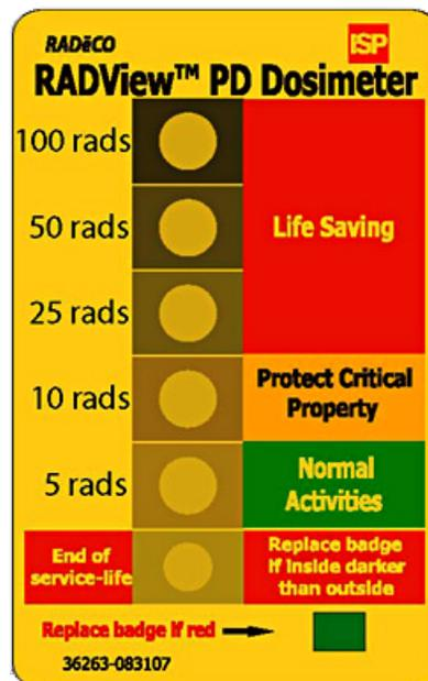
**Figure 3** Gamma radiation dosimeter (left) in chamber, (right) badge
