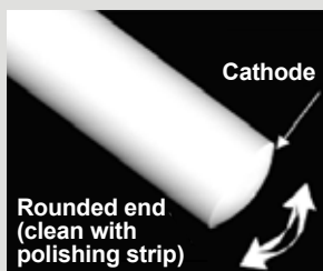
Figure 4 Cleaning a contaminated cathode by pressing the green polishing strip lightly against the glass and turning it 10 to 20 times.
