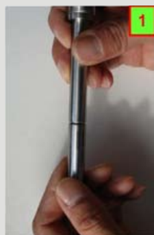
Figure 5 Electrode replacement procedure: unscrew the old membrane cap, fill with 1.5 ml of electrolyte solution, and screw on new membrane cap.
