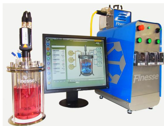
Fig. 1: Picture of the novel glass bioreactor together with Finesse TruViu RDPDmini control system
