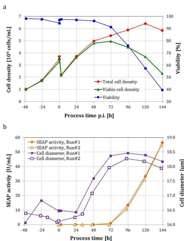
Fig. 2: Offline-data of the *Sf-9* insect cell culture in the «SmartGlass» bioreactor (a) Total and viable cell density and viability, (b) SEAP activity and average cell diameter.
