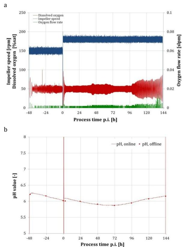
**Fig. 3: Online data of the *Sf-9* insect cell culture in the «SmartGlass» bioreactor. (a) The impeller speed, dissolved oxygen level and O<sub>2</sub> flow rate used for the DO control, (b) Comparison of online measured pH values with offline analyses. The virus infection was realized at 48 h of cultivation, which can easily be identified by the peak in the pH profile resulting from the disconnection of the pH probe from the control unit.**
